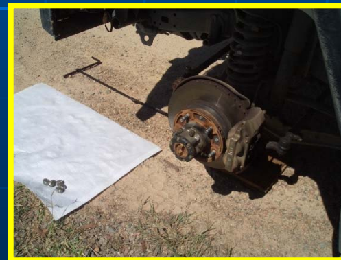
Remove all Wheel Nuts and take off Wheel.
