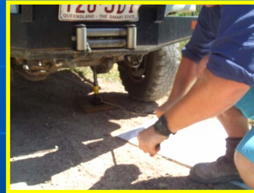
Lift Vehicle high enough with Jack
