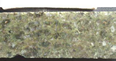
Figure 52b. Strongly green Sericite Altered Granite basement
