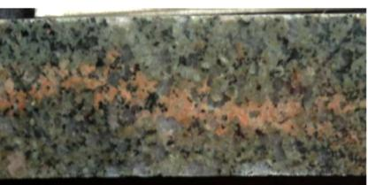
igure 53a. K-Feldspar veinlets cutting sericite Iltered granite basement
